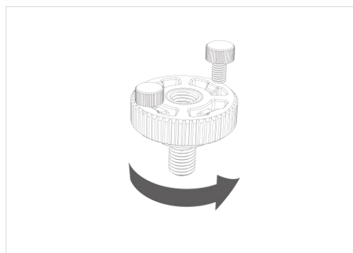
Pic.13. Using two small bolts as leverage.
