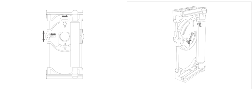
Pic.12. Installing the Blinder to cover the back of Viewing Circle.
